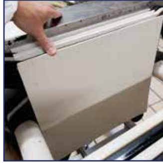
Step 4 Insert the fourth sheet in the opposite direct with respect to the sheet previously inserted.
