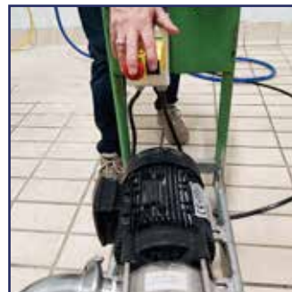
Step 12 Start the pump again at a speed 1.5 times faster than the filtering speed for about 5 minutes.
