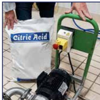
Step 11 Stop the pump and add citric acid to the washing water.
