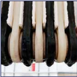
Step 7 Make sure that the sheet is not "pinched" between the gasket and the frame.
