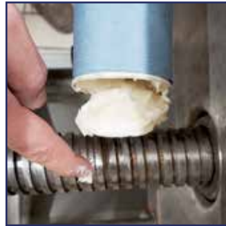
Step 8 Lubricate the worm screw (this should be done periodically).
