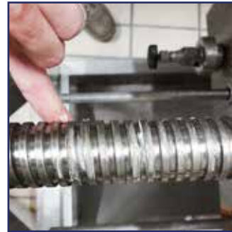
Step 8 Lubricate the worm screw (this should be done periodically).
